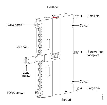
The T-10 TORX driver tool and a 1/4-inch flathead screwdriver are used to remove and install the cable bar clamp on the UCH, and loosen the line card captive screws.
